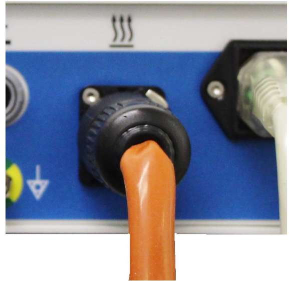
Figure 9: Plug Heater Band Cord into Receptacle
