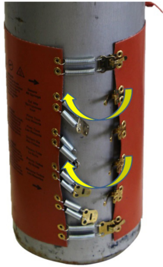
Figure 8: Secure All Tensioning Spring Retainers
