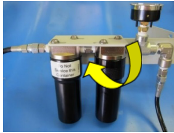
Figure 23: Filter Housing Removal
