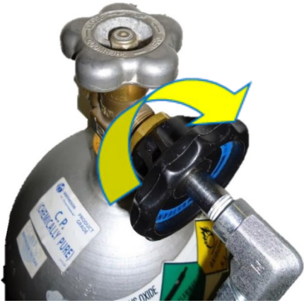
Figure 5: Attach Black Knob to Threaded Connection
