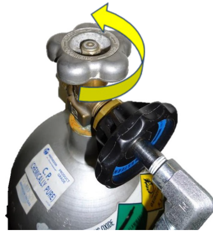
Figure 6: Turn Valve Counter-Clockwise to Open
