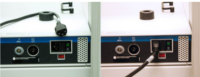
Figure 31: Insert the power cord into the power entry module of the cryoICE BOX.
