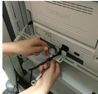
Figure 71: Install the Printer Cable Bracket on the AC Power cable.
