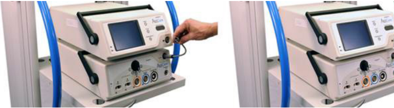
Figure 10: Installation of the Hand Piece Jumper Cable between the ASU and ASB.
