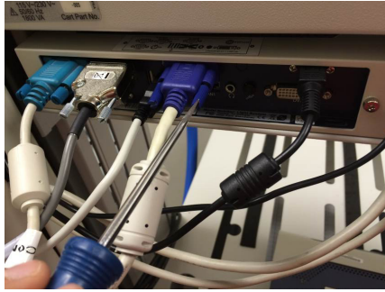
Figure 59: Tightening the thumb screws, required on the Video, COM1, and COM2.
