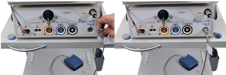
Figure 11: Connect the Footswitch Cable to FOOTSWITCH connector on the ASB.
