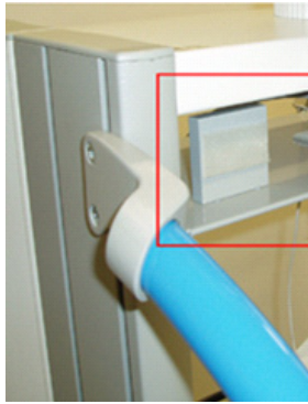
Figure 62: Metal tab with Velcro strip- located on the top shelf of the ORLab System cart
