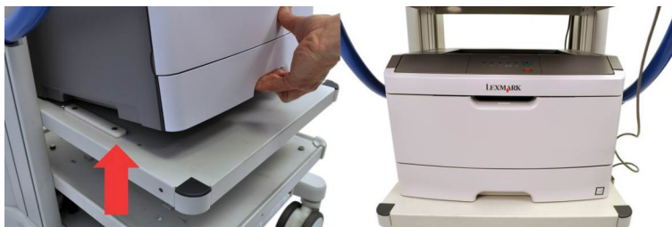
Figure 69: Line up with the brackets mounted on the top of the Printer Shelf with the handle recesses on the bottom of the printer.
