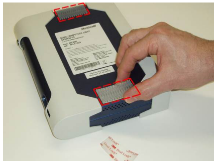
Figure 55: Apply two Velcro strips to the outside edges of PC Housing.
