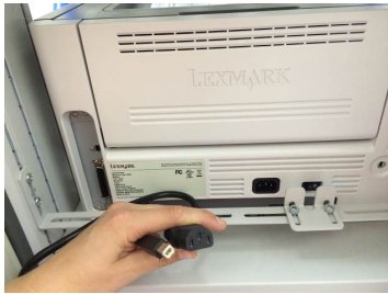
Figure 70: Attach Printer Cable and Power Cable to rear of printer.
