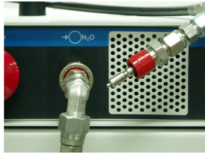
Figure 36: Align the quick-connect gas connector with the cryoICE BOX N2O inlet port. Insert and push in the connector until you hear it “click”.
