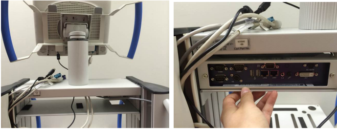
Figure 56: Mount the MicroPace PC on the left side of the top shelf.
