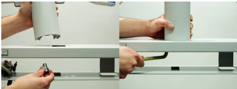
Figure 40: Mount the Monitor Holder from the rear of the Basic Cart.
