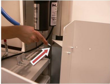
Securing Right Tank Holder
