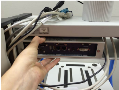
Figure 57: Apply firm pressure to the top of PC (near the edges) until securely attached.
