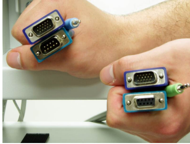
Figure 41: Monitor cables: Monitor end (right hand) and PC end (left hand).
