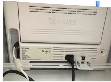
Figure 70: Attach Printer Cable and Power Cable to rear of printer.
