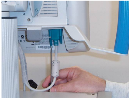
Figure 54: Mounting screws on the Video and Serial Cables must be tightened using a flat head screw driver.
