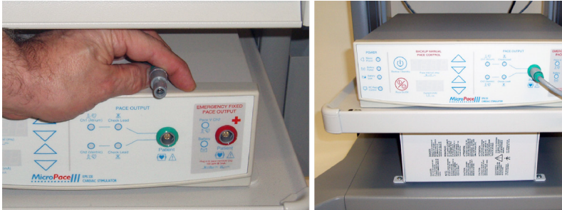
Figure 73: Connect the Pace Output Cable to the 'Patient' connector on the front of Stimulus Generator.
