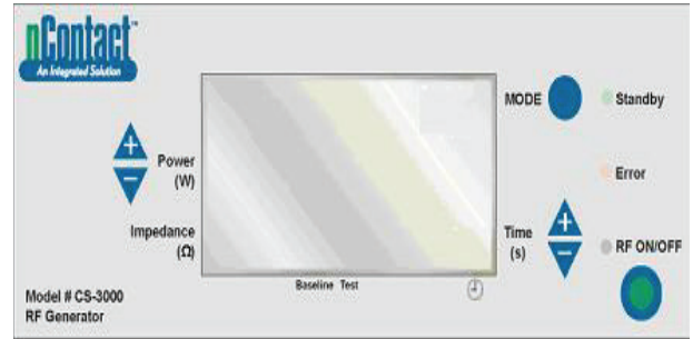
Figure 8. RF Generator Front Panel Display at “Power On”
