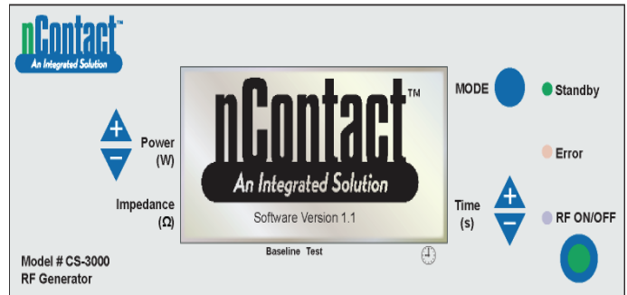
Figure 9. RF Generator Front Panel Display at “Standby Mode”
