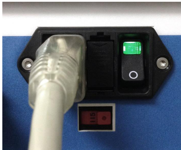
FIGURE 10: TURN-ON ATRICURE CRYOICE BOX WITH SWITCH
