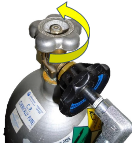
FIGURE 6: TURN VALVE COUNTER-CLOCKWISE TO OPEN
