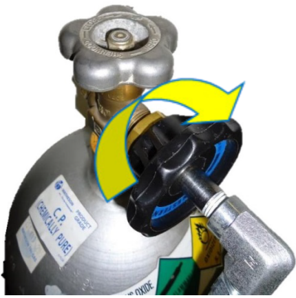
FIGURE 5: ATTACH COUNTRY SPECIFIC COUPLER TO THREADED CONNECTION
