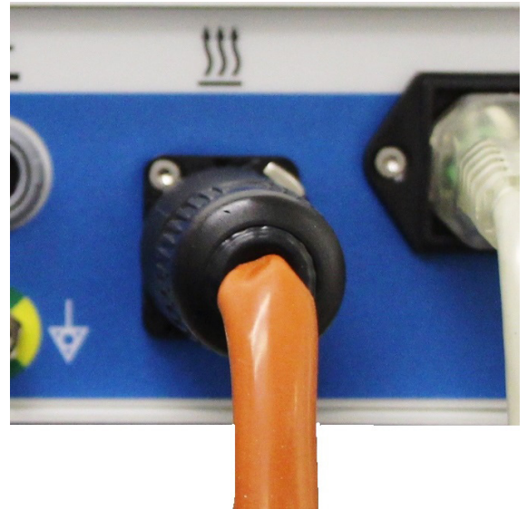
FIGURE 9: PLUG HEATER BAND CORD INTO RECEPTACLE
