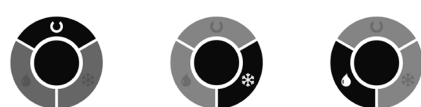
[a] Ready Mode (green) [b] Freeze Mode (blue) [c] Defrost Mode (orange)
